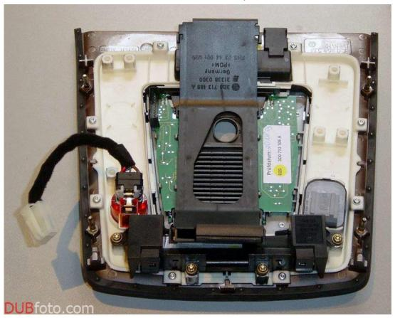
**4.4** Remove the cigarette lighter assembly from its hole is a real \*\*\*\*\*\*, so go carefully. Locate the two orange tabs inside lighter hole and gently releasing them by pressing a small screwdriver into each one. This will let it slide out of the orange styrene surround and the process of getting it out of the trim panel goes like this:
