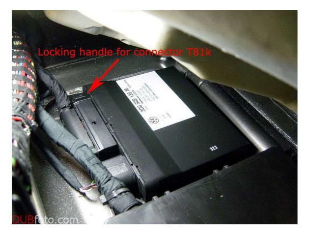
**5.8** At this point, I am going to refer you to Spockcats website, <u>Touareg Keyless Start Install Instructions</u>, where he details the process of doing the same thing on a Touareg. The Touareg has the same connector and same access/start control module, it is just located in a much easier position to get at in the Touareg.
