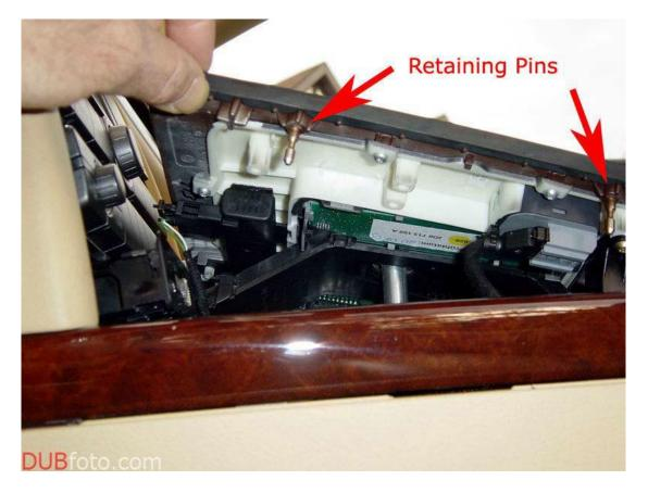
Remove the connectors on the left side (mirror control) and the aft end (seat heating, ESP, etc.) first, then you can lift the panel up and over the transmission select post, and turn it upside down. This makes it much easier to separate the connector that supplies power to the cigarette lighter. That particular connector requires quite a bit of force to get apart.
