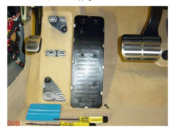
**5.6** (This step is difficult and can be frustrating.) Starting at the forward, top, outboard area of the driver footwell carpet, above the deadpedal area, pull the carpet back and downwards, and fold it under the brake pedal, so that that whole area of the carpet is now covering up the brake pedal (in other words, towards the rear of the car, not towards the front of the car).
