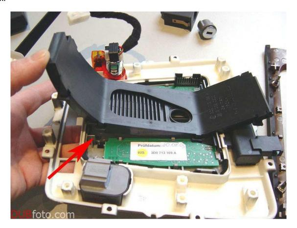
**4.6** Remove the chrome surround for the transmission select lever by releasing the two tabs that hold it in place. Once you have this part out, you will see 4 little self-adhesive fabric strips in each corner of your "old" grey trim piece. Carefully remove these, and put them in the same locations on your "new" trim piece. They stop the metal assembly from squeaking against the plastic.
