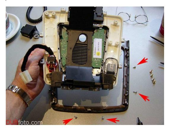
**4.2** Remove the mirror adjustment switch. Use a jeweler's screwdriver to loosen the small plastic retaining pins, and just push it up from underneath.
