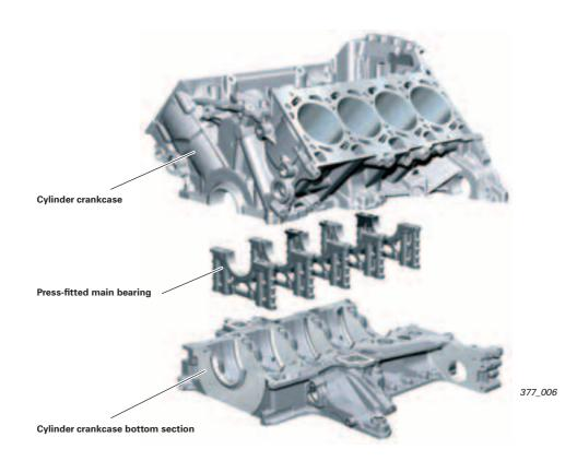
The cylinder crankcase lower section (bedplate bearing cross-member) is made of aluminium with press-fitted iron main bearing covers made of grade 50 nodular cast iron. It is centred using centring pins, sealed with liquid sealant and bolted to the cylinder crankcase.
