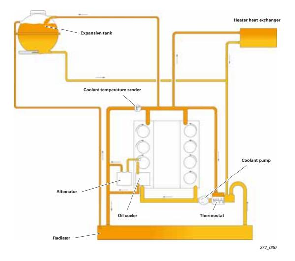
The cooling system in the new V8 engines was configured as a longitudinal-flow cooling system. The cooling water flows in on the outlet side and through the cylinder head gasket into the cylinder head, where it flows out longitudinally through the chain housing cover.
