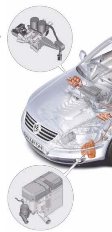
Auxiliary/supplementary heater with control unit, front left beneath wing
