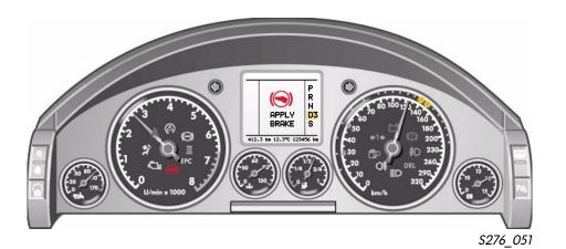
The LED ring around the speedometer and the red symbol for the APC in the rev counter are redundant and provide the minimum necessary information to the driver in case the colour screen is unavailable.
