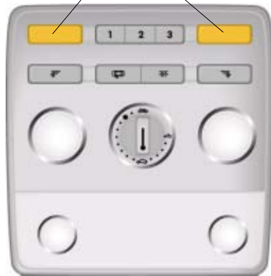
Front roof module
