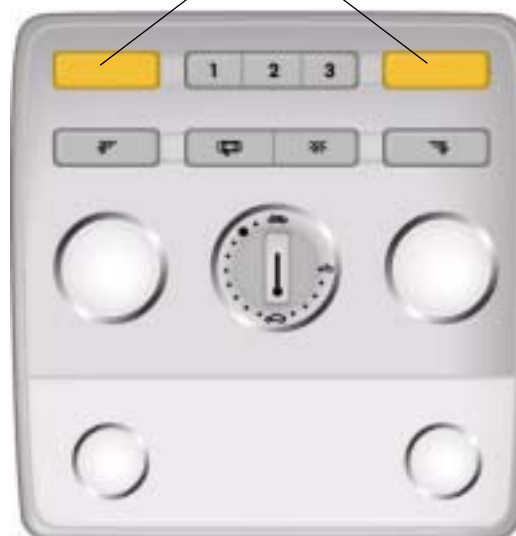
Front roof module
